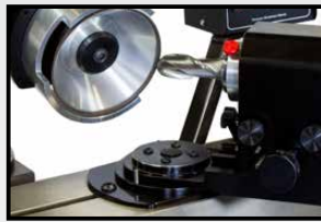
Bull Nose / Ball Nose Corner Radius
