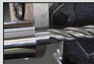
Reduced Neck and Weldon Flat Grinding
