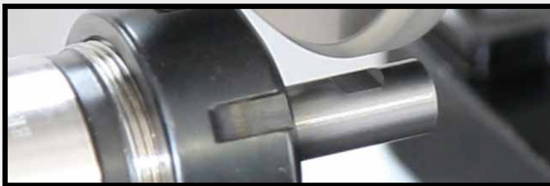
Set Screw Flat, neck Reduction and carbide cut off
