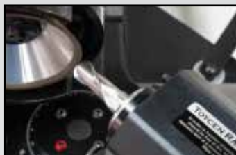
Corner Radius (Bull and Ball Nose )
