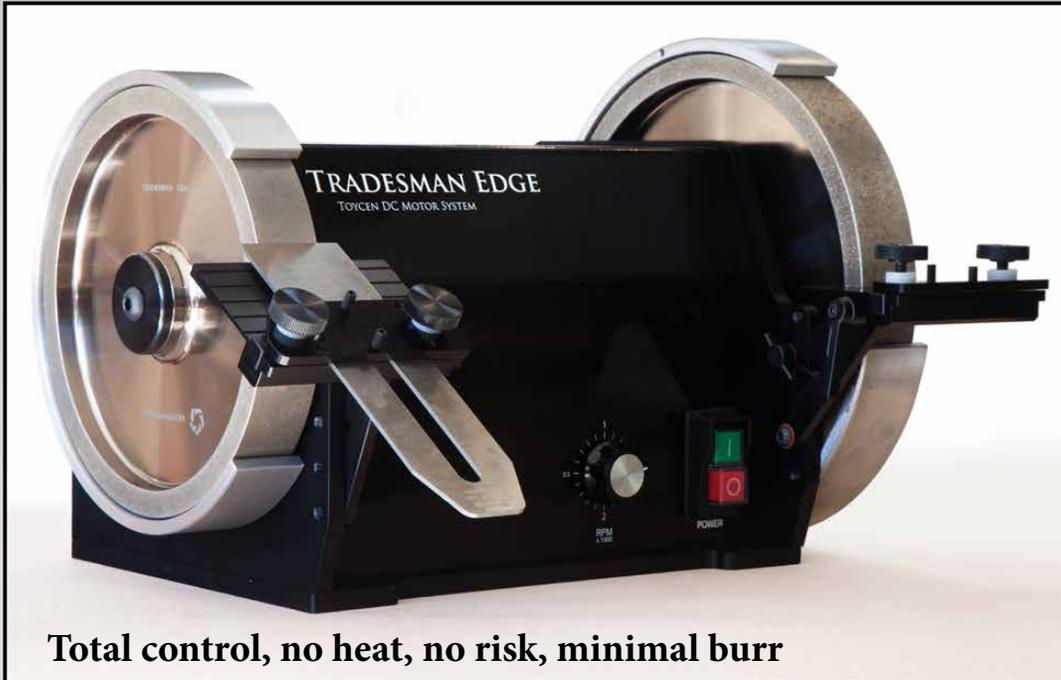
The Motor is shaft is isolated from the main shaft with a geared timing belt, the main shaft is 1" diameter, uses the same large single row ball we use in our largest tool grinder. ToyCen DC whisper drive Speed ranges from 150 to 3000 surface feet and is reversing. Yes, you can stand a coin on edge on top of the machine at any speed range (the Tradesman Loonie test). Smooth is the name of the game. Reversing, quiet, and unstoppable geared belt drive, available in various speed ranges.
