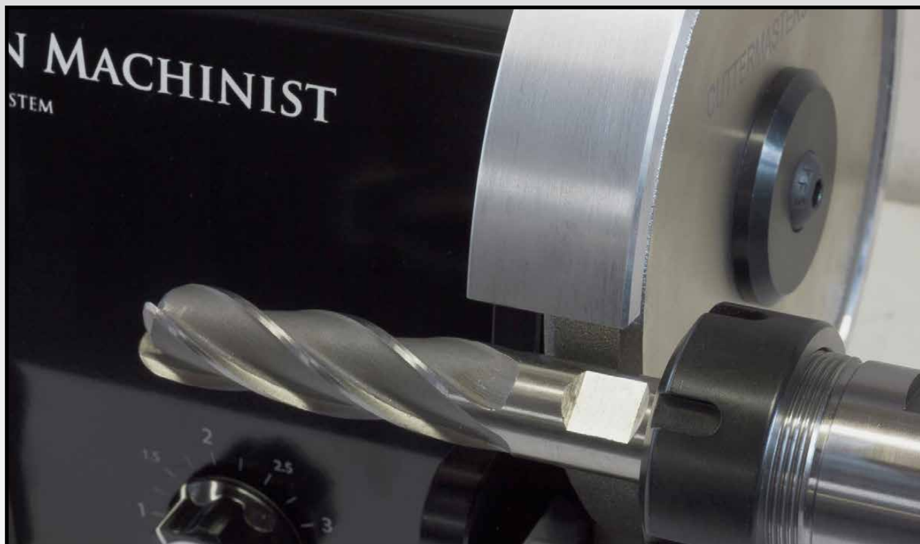
Grinding a Weldon Set Screw Flat. Tradesman Machinist with CM-WF.5 Weldon Flat Wheel
