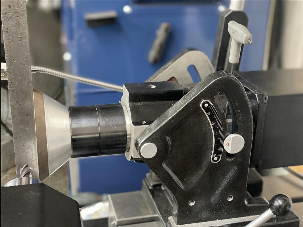
Grind the primary angle, watch your indicators. Go as close to center as you can with out taking the tips off the corners
