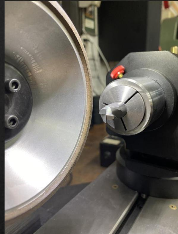
Feed across the tool at a good rpm and an even rate
