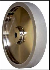
Our square cornered 8" grinding wheels have a full width of 1.27", 1/2" plated side flange, and 5/8" arbor. The square corners have a small radius to maintain plating strength. These wheels are available in four grits:
