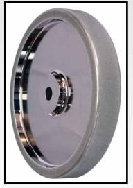
Our round cornered 8" grinding wheels have an over-all width of 1.30", a flat width of 0.98", 1/2" plated side flange, and 5/8" arbor. The rounded corners have a 0.16" corner radius. These wheels are available in four grits:
