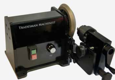
Tradesman Neck and Cut Off with the T-SDC Step Drill and Countersink Attachment
