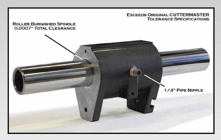
The CM-02A Air Spindle Upgrade for CUTTERMASTER and CUTTERMASTER type machines replaces the main body and spindle of the air bearing. It is an improvement over the original air bearing supplied with the CM-01 and MG-30 CUTTERMASTERs, in that the bushing is roller burnished and provides greater tolerance (0.0007").
