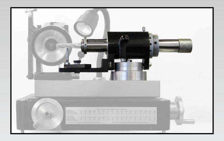
The CM-02 Air Spindle for CUTTERMASTER and CUTTERMASTER type machines is a fluid air bearing that floats on a cusion of air when air is applied. This is what allows the operator to create helical grinds, like the outside diamter of an end mill or router bit. It is an improvement over the original air bearing supplied with the CM-01 and MG-30 CUTTERMASTERs, in that the bushing is roller burnished and provides greater tolerance.
