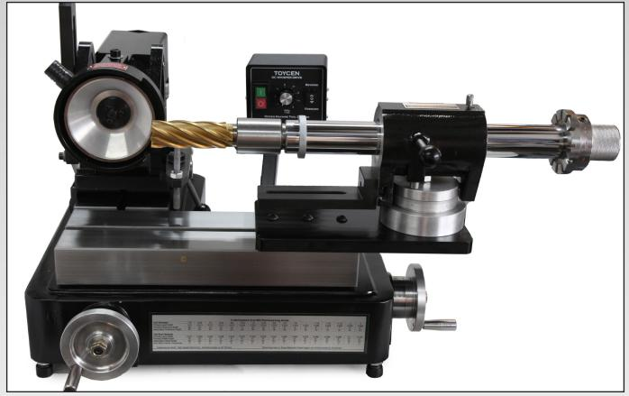
Increase the maximum flute length of the Journeyman End Mill Grinder with the JX-XAE X-Axis Extension Kit. By mounting the stylus to the motor, and extending the x-axis way, flute lengths of up to x" are acheivable. This kit includes the JX-Riser and requires the Journeyman motor, which unlike the original CUTTERMASTER motor, can pivot.
